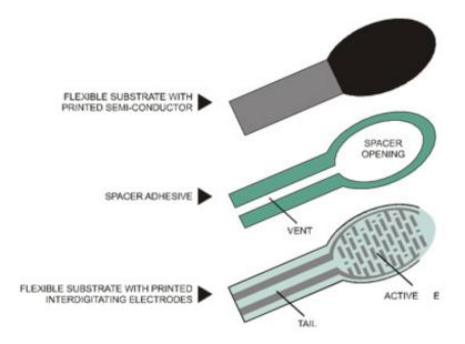
FSR's are basically a resistor that changes its resistive value (in ohms  $\Omega$ ) depending on how much its pressed. These sensors are fairly low cost, and easy to use but they're rarely accurate. They also vary some from sensor to sensor perhaps 10%. So basically when you use FSR's you should only expect to get *ranges* of response. While FSRs can detect weight, they're a bad choice for detecting exactly how many pounds of weight are on them.
