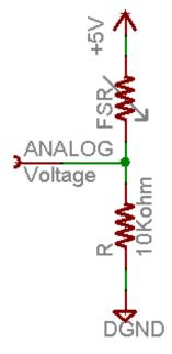
For this example I'm showing it with a 5V supply but note that you can use this with a 3.3v supply just as easily. In this configuration the analog voltage reading ranges from 0V (ground) to about 5V (or about the same as the power supply voltage).
