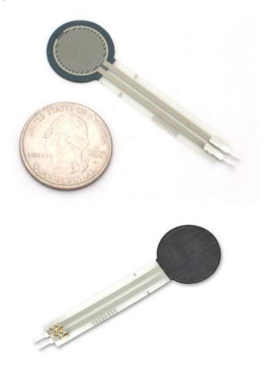
The FSR is made of 2 layers seperated by a spacer. The more one presses, the more of those Active Element dots touch the semiconductor and that makes the resistance go down.
