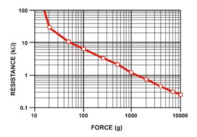
Its important to notice that the graph isn't really linear (its a log/log graph) and that at especially low force measurements it quickly goes from infinite to  $100 \mathrm{K}\Omega$ .
