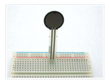
FSRs are often a polymer with conductive material silk-screened on. That means they're plastic and the connection tab is crimped on somewhat delicate material. The best way to connect to these is to simply plug them into a breadboard.
