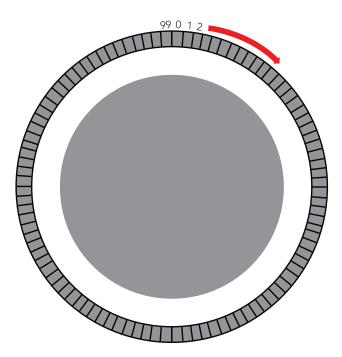
The onboard data logger can be programmed to store readings at an interval as small as once every 10 seconds and as large as once every 320,000 seconds (3.7 days). The onboard data logger stores the readings in a circular buffer beginning at memory location 0.
