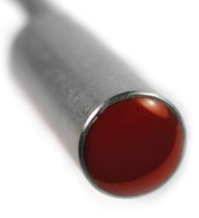
The bottom of the sensor is made of a high viscosity moderate porosity epoxy. This moderate porosity epoxy is further encased in a low viscosity no porosity red epoxy. This allows for high temperature and pressure resistance, as well as being 100% water impermeable.
