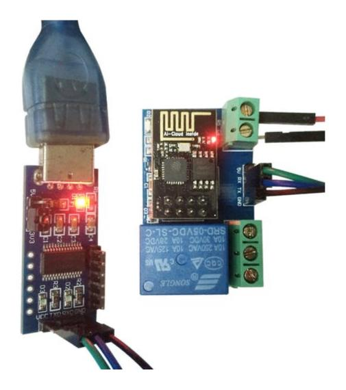
3. The default Baud rate of the WiFi module is maybe 115200 or 9600. You can send AT commands to change it, such as: AT+CIOBAUD=115200. I recommend you use 115200 in general conditions, but you should change it to 9600 when you use a cell phone to control the relay (because the Baud rate of the onboard MCU STC15F104W is 9600).
