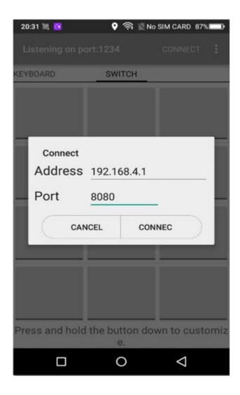
• Press the function blocks and enter the name and content of the serial command (A00101A2 open relay, A00100A1 closed relay, command format must be hex).
