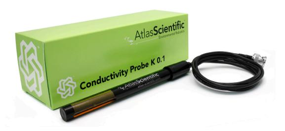
This Atlas Scientific conductivity probe, has a cell constant of **K 0.1** When this conductivity probe is connected to an Atlas Scientific EZO<sup>TM</sup> conductivity circuit, it has a range of **0.5**  $\mu$ **S/cm to 50,000**  $\mu$ **S/cm**
