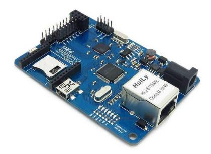
The Iboard Ex is a unique Arduino board which features a WIZnet Ethernet port with POE, an XBee socket, nRF24L01+ module interface, Micro SD socket and an ATMEGA32U4. This board will add wireless XBee control as well as internet connectivity to your projects. And don't need any external programmer, just connect it with PC by a USB cable. It's great for anything from home automation to robot control. The possibilities are endless!
