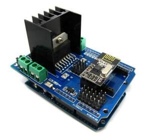
MotoMama is an H-Bridge motor driver shield bases on ST L298N chip. It is a high voltage, high current dual full-bridge driver which designed to accept standard TTL logic levels and drive inductive loads such as relays, solenoids, DC motor and stepping motors. MotoMama is designed to be easy with other sensors or wireless modules.
