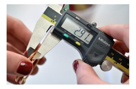
The coils should be 3mm or closer for most efficient energy transfer.
