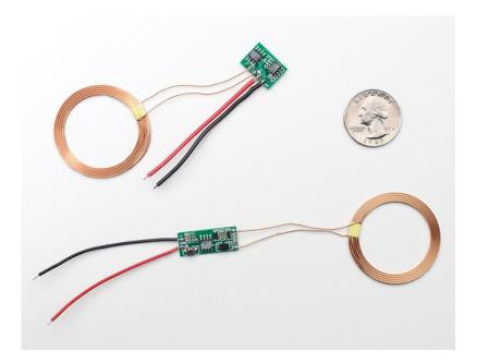
Inductive charging is a way of powering a device without a direct wire connection. Most people have seen inductive charging in a rechargeable electric toothbrush: you may have noticed that you recharge it by placing it into the holder, but there's no direct plug. These chargers work by taking a power transformer and splitting it in half, an AC waveform is generated into one, and couples into the second coil.
