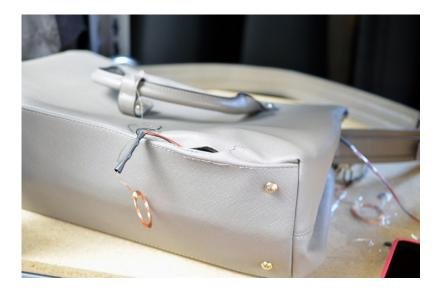
Open the bottom of the bag with a seam ripper, and run the USB cable up into the chamber of the purse. Plug it into your phone or battery pack, and slide the induction coil behind the very outer layer of fabric/leather/etc. Tip the bag upright, align with your magnets, and play around with the position of the coil until the two line up and your phone is charging! Tape it in place inside the bag.
