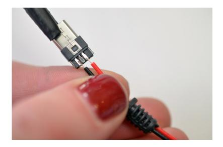
The red and black wires affix to the outer pads on the USB connector as shown above. At this point you may wish to lengthen the wires attached to the long skinny circuit board to give your USB cable some slack inside the bag. When you've got wires of your desired length in place, slide on the strain relief collar that comes with the USB connector.
