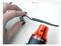
Cut off the barrel connector from the AC adapter, and strip the red and black wires inside. Slide a medium diameter piece of heat shrink tubing over the whole wire, then put a smaller piece on each of the two wires.
