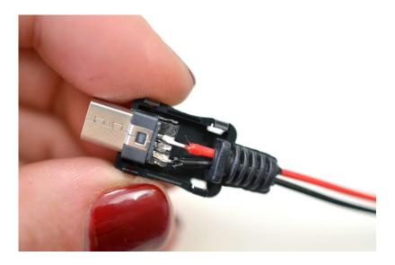
Close up the USB connector by placing the port and strain relief collar in one half of the plastic shell.
