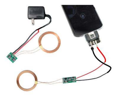
Reference the above circuit diagram when building this project! The coil attached to the more square circuit board attaches to the incoming power, in this case from a 9V AC adapter. The other, more long and skinny, circuit board gets soldered to the USB connector as shown.
