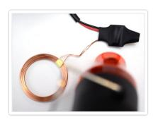
Use a large piece of heat shrink tubing to protect the circuit board. Repeat with the coil assembly that will go in the bag.
