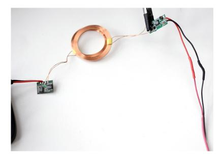
It's time to test your circuit! Plug the AC adapter into the wall and use helping hands or other things on your desk to orient the coils as close as possible to one another. They must be coaxial (parallel).
