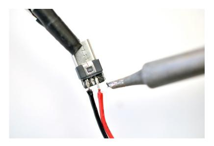
With the help of a 3rd hand tool, tin the pads and wires separately and then reheat with your soldering iron to make the connections.
