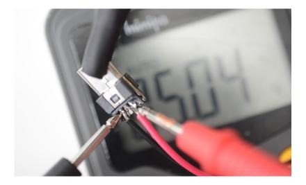
With the coils in place, use a multimeter to test the output on the USB end. It should read 5 volts.
