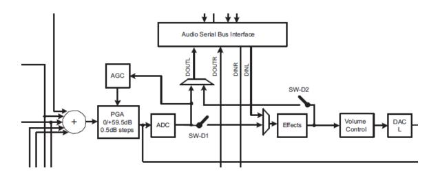
Figure 4. The Record Path of TLV320AIC3106
