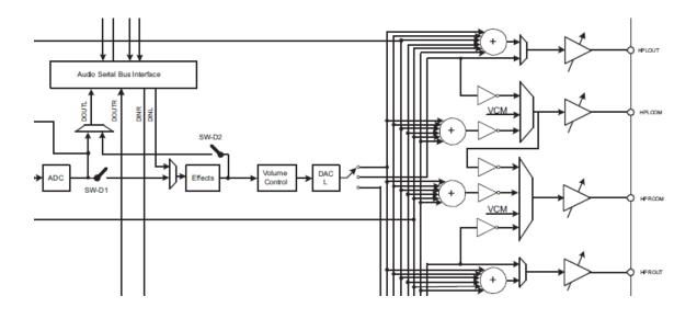
Figure 5. The Playback Path of TLV320AIC3106
