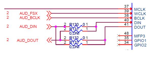
Figure 6. Audio Serial Bus Interface
