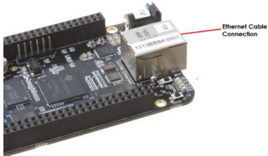
Figure 12. Ethernet Cable Connection
