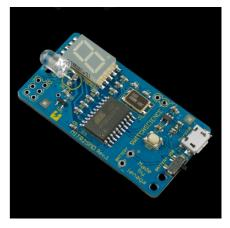
Please solder the IR LED onto the board. The location is marked as "IRLED". The LED has two leads, longer and shorter. The shorter lead should be inserted into the hole nearer by the "IRLED" marking. The IR remote will not work if you solder with wrong holes.
